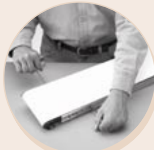
Adjust tension on new belt, tighten fasteners and go!
